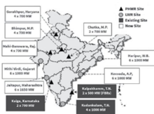
FIGURE 2. Location of the sites in India where indigenous PHWR 700 & FBRs and the imported generation III + LWRs have been planned.
